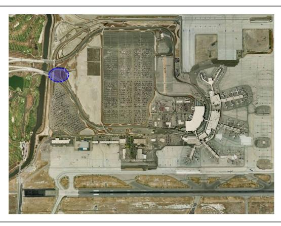
**Project Description:** This project is part of a continuing program to maintain the Airport's infrastructure. This project will consist of the construction of an asphalt overlay on 2100 North and 4000 West streets from the intersection of 2200 West to the intersection of 1200 North. Work will include asphalt milling, installation of new bituminous surface course, and pavement markings.
