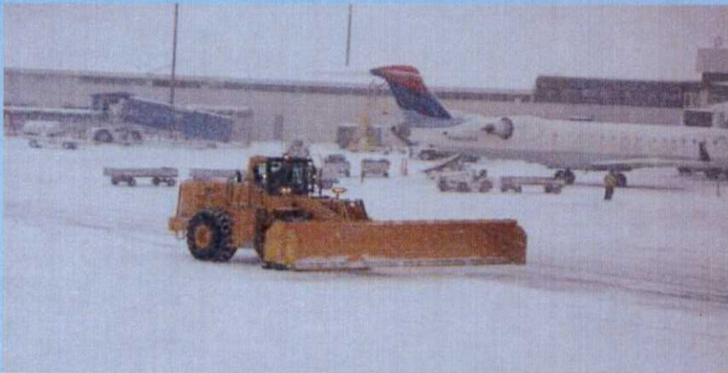
375 Horsepower Front End Loader with 30' Plow
