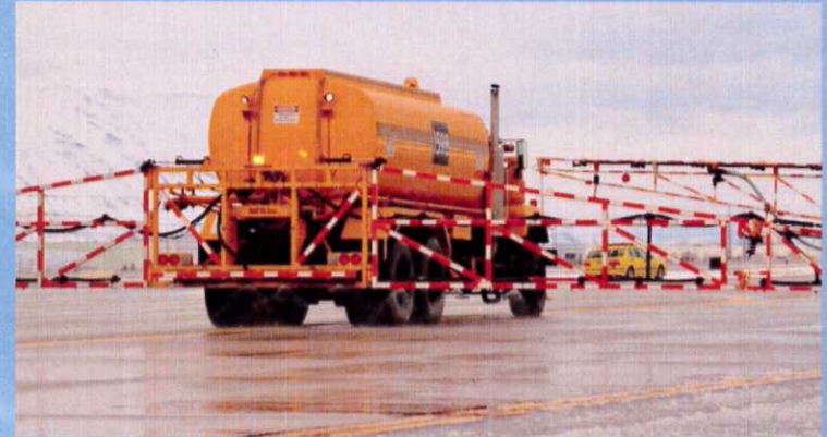
4,800 Gallon Liquid Deicer Truck with 75' Wide Spray Boom
