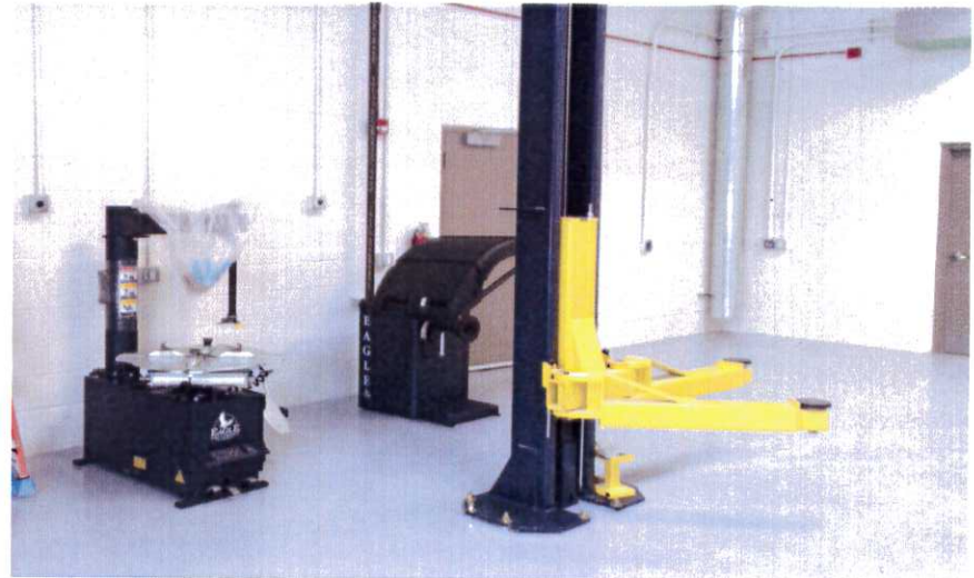
RSS 'A' tenant car care equipment and epoxy floor coating
